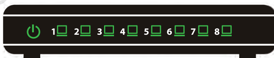
Figure 5.8: A network hub with 8 ports
